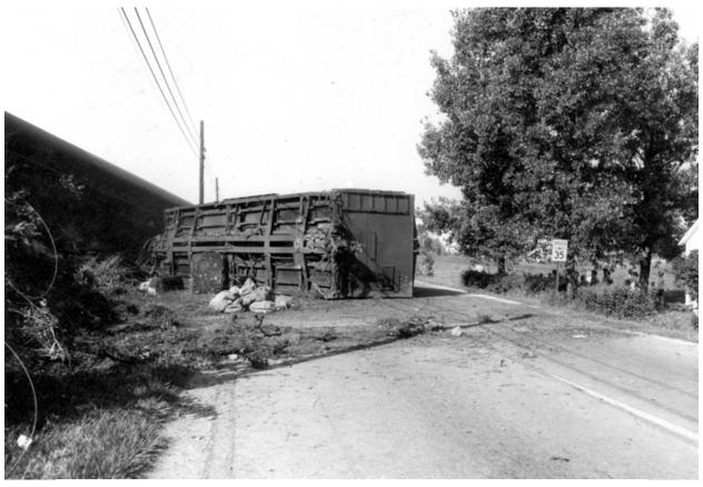
Rough track and poor truck maintenance on the box car preceding this one started the trouble. The box car rocked off the track and one of its trucks turned 90 deg pulling up the track spikes as it went along. That spread the track causing all the following cars to derail. The box car following the offending car ended up in the middle of Rt. 142. The Pullman car that was following it was left on the embankment as shown above. Photo by Dave Bunge.
