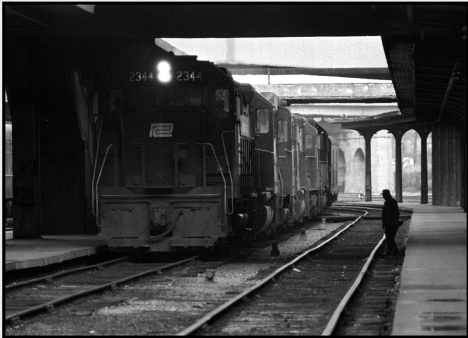
On another day, a westbound mail train creeps down Track 3 and yet another round of switching will occur. Tight times on the PC are evident in the missing MU cables on the lead unit - undoubtedly scavenged for use on other units.
