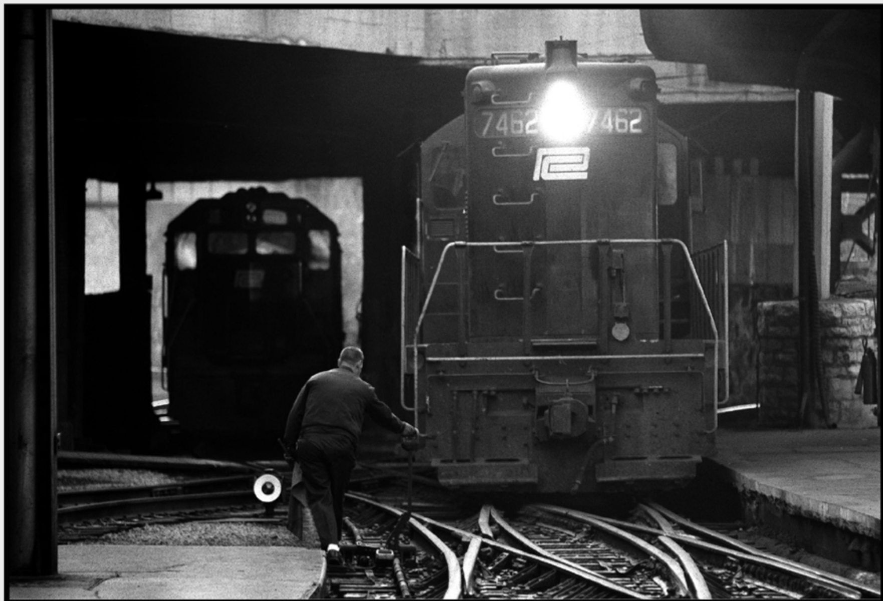
The station switcher, under the careful gaze of the mail train road power in the background, prepares to reach down Track 2 and grab two Flexi-Van cars full of local mail. One of several station switchmen throws a 'puzzle' switch in preparation for the move.
