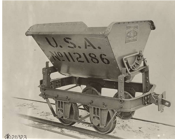
Kilbourne and Jacobs "V Skip" wagon awaiting delivery to the U.S. Army, 1917 (photo made available by Creative Commons)
