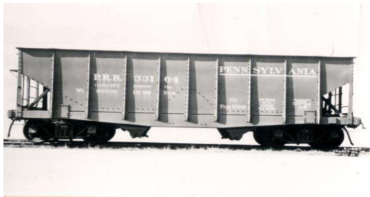
50-ton two-bay steel hopper built by Schoen Pressed Steel Car Co., McKees Rocks, PA, in 1898, https://explorepahistory.com/displayimage.php?imgId=1-2-68C
