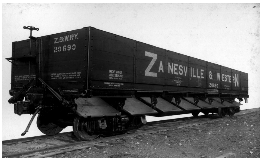
A 1907 Ralston drop bottom gondola built for the Z&W
