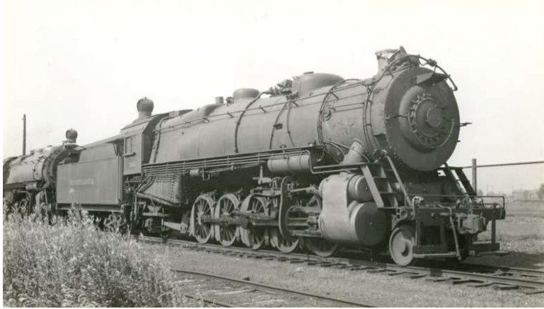
PRR N2sa 2-10-2 No. 7937 in storage, 1935. Once the Great Lakes shipping season ended each year, a portion of PRR's Lake Region heavy engines would be laid up until the following spring. Photo by J.H. Dean from Alex Campbell Collection.
